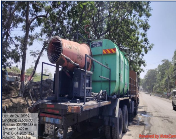
Fig:- Water Sprinkling on Road via truck mounted Smog-Gun
